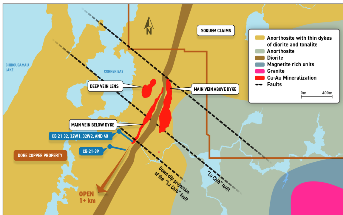
Figure 4. Geology map of the Corner Bay deposit with projections to surface of the potential mineral resources of the main vein defined in the 2019 NI 43-101 Technical Report and showing location of hole CB-21-32 and 32W1 (assays received).
