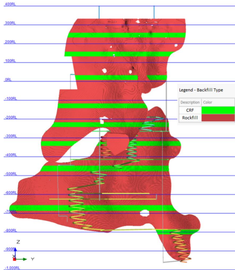
Figure 16-18: Backfill type – Corner Bay (long section looking west)
