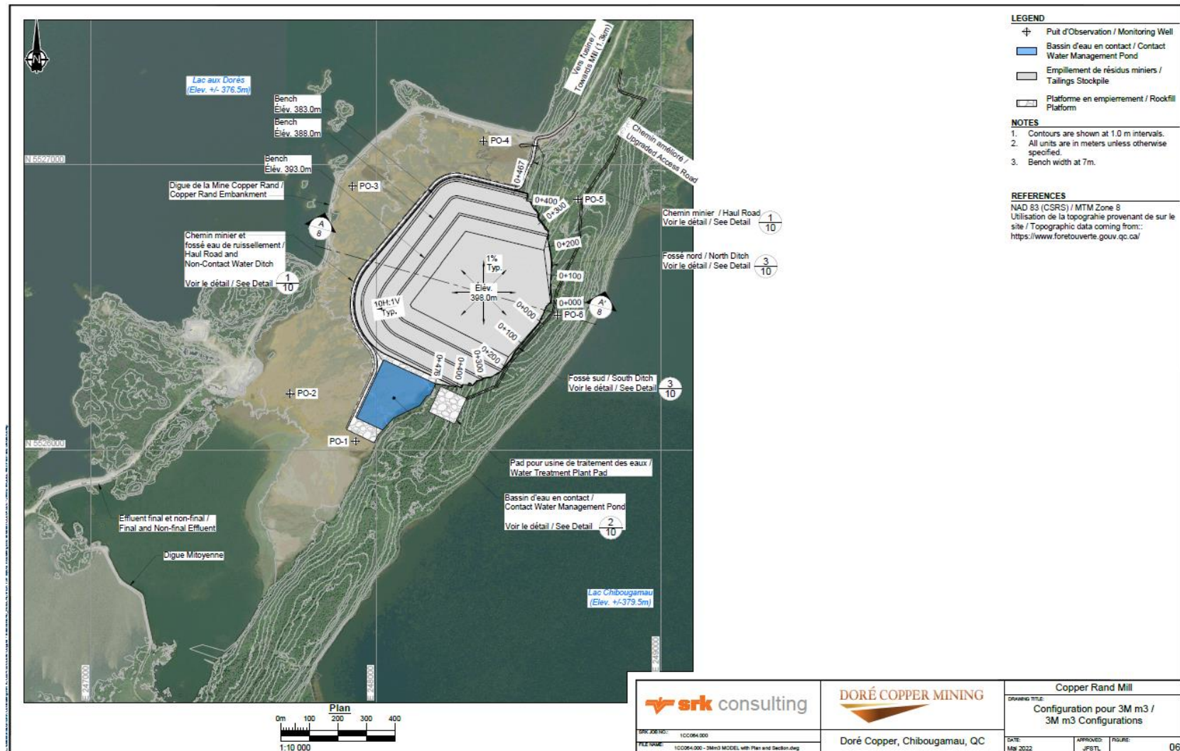
Figure 18-13: TMF configuration at end of LOM
