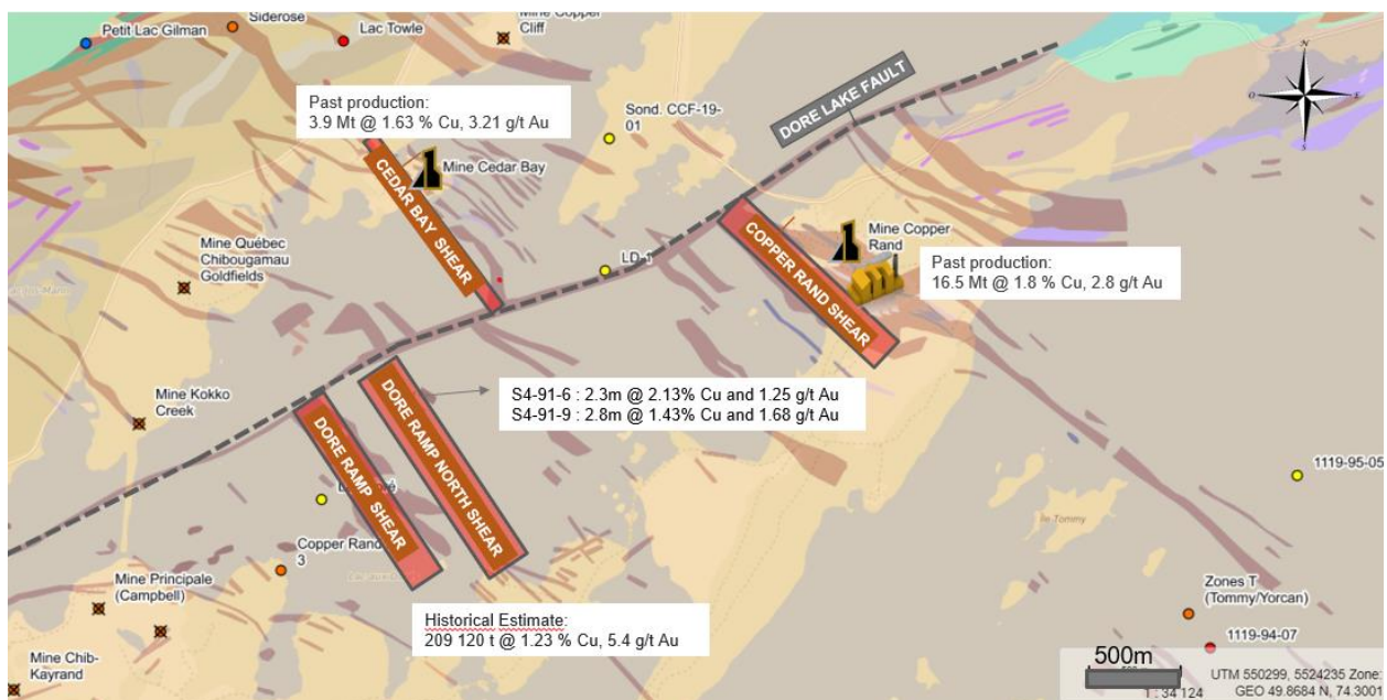
Figure 1. Location map of the Doré Ramp and Doré Ramp North shear zones with respect to the past producing Copper Rand mine and mill and Cedar Bay mine.
